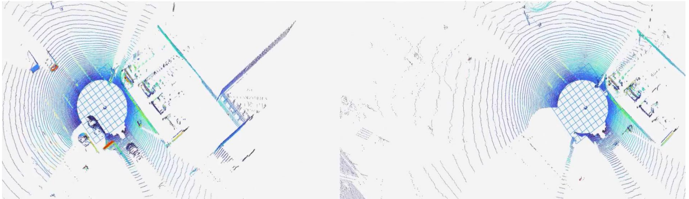
Figure 8: Example of the AI-based dynamic object removal applied to LiDAR scans. Left: Raw LiDAR point cloud including moving objects such as cars [7]. Right: Filtered point cloud after applying the proposed algorithm, where dynamic features have been removed, leaving only static features for robust localization and mapping.
