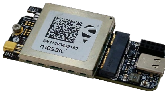
Figure 3 M.2 Mosaic GNSS receiver board with USB-C Interface board
