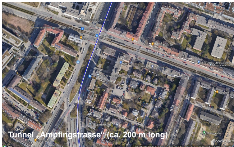
Figure 5: Passage through the tunnel Ampfingstrasse with a length of 200 m. The ANavS solution closely follows the reference solution within the tunnel. There is no drift nor jump visible at the start and end of the tunnel.
