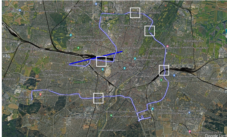
Figure 4: Map with trajectory of test drive in Munich, Germany. The test drive follows the interior highway circle (B2R) for most of the time. The white trajectory corresponds to the ANavS solution. The blue trajectory corresponds to the RT3000 OXTS solution, which serves as reference. The track includes several tunnels with lengths ranging from a few hundred metres to almost 2 km. Some tunnels are highlighted by the white boxes.
