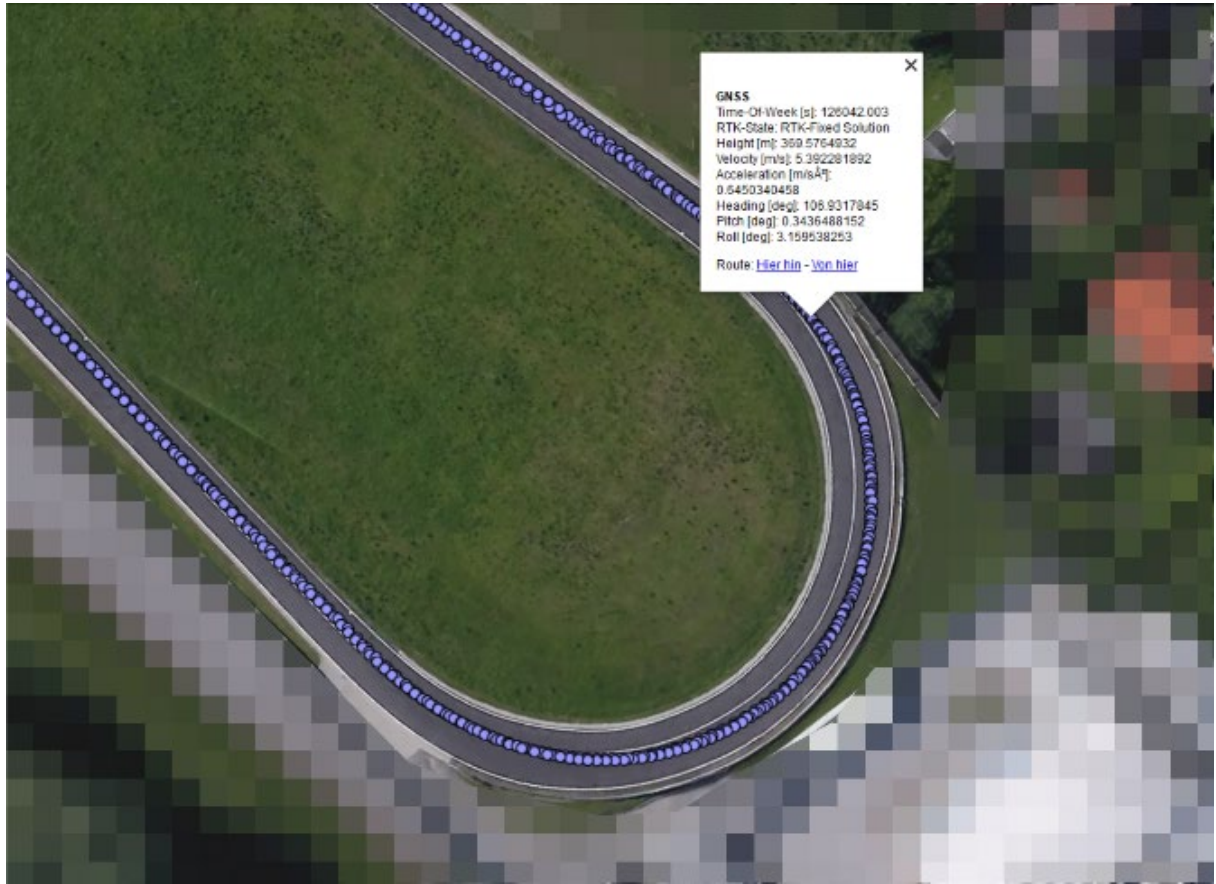
Figure 58: Example kml-file where each purple dot is showing the most interesting states like position, velocity, acceleration, and attitude.
