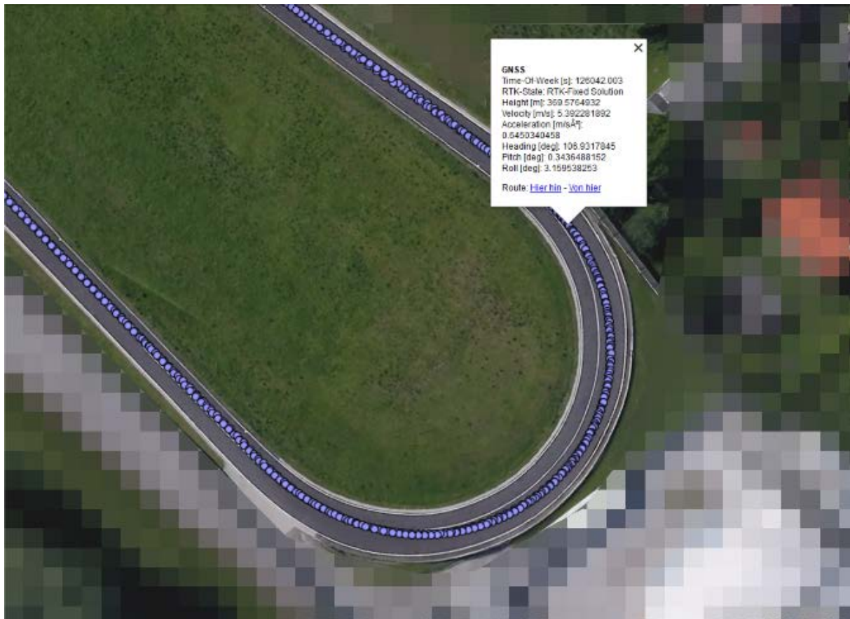
Figure 42: Example kml-file where each purple dot is showing the most interesting states like position, velocity, acceleration, and attitude.
