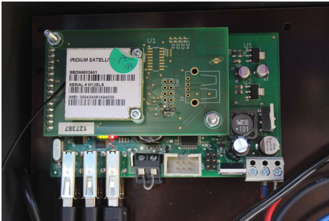
Figure 2. Processing board with integrated snow parameter estimation, power management unit and satellite communication module.
