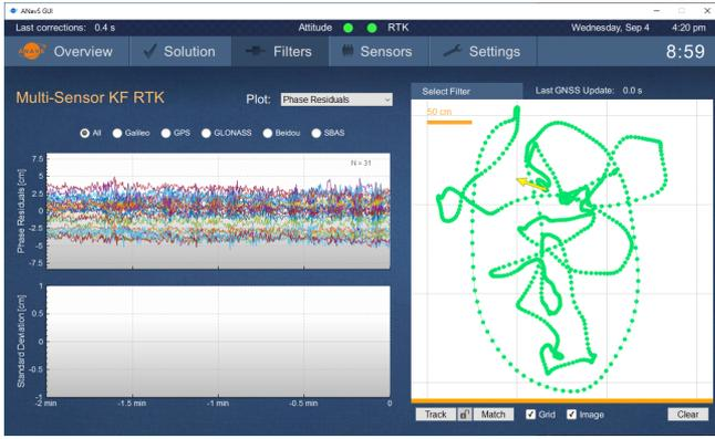
Fig. 4. Ground-track of UAV as shown on ANavS GUI. The left subfigure includes the fixed phase residuals; each line/ color refers to one satellite. The right subfigure shows the ground-track on a map. The noise levels of both the residuals and the position track are in the order of only 2 cm.
