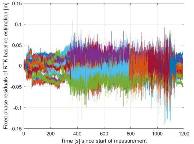
Fig. 9. Fixed phase residuals of RTK baseline estimation for all used GPS, Galileo, GLONASS and Beidou satellites. The residuals are for all satellites for most of the time below 5 cm, which indicates the accuracy of the position solution.
