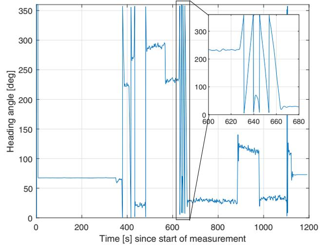
Fig. 6. Heading of UAV during test flight. The enlarged section in the upper right corner shows the heading during the turning of the UAV.
