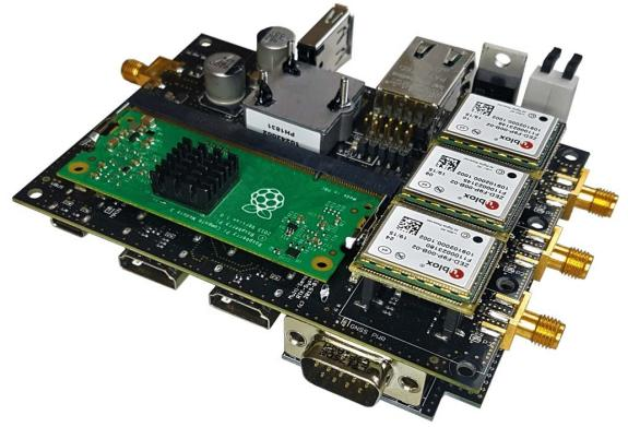
Fig. 3. Photo of Multi-Sensor Real-Time Kinematic (MS-RTK) positioning module of ANavS: The module includes 3 Multi-GNSS, Multi-frequency receivers for accurate position and attitude determination, an industrial-grade MEMS IMU, a barometer, a GSM/ LTE module for the reception of RTK corrections, a processor for running the RTK positioning with a tightly coupled sensor fusion and various other interfaces for additional sensors.
