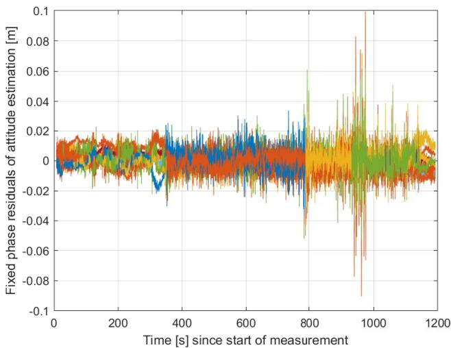
Fig. 8. Fixed phase residuals of attitude estimation for all used GPS, Galileo, GLONASS and Beidou satellites. The residuals are for all satellites for most of the time below 2 cm, which indicates a correct ambiguity fixing.
