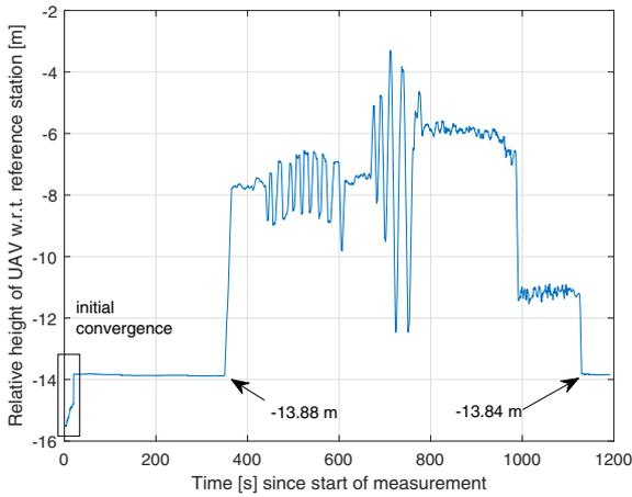
Fig. 5. Height of UAV relative to reference station.
