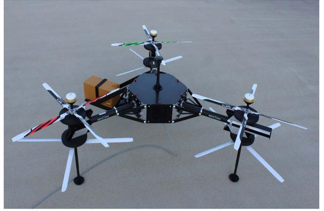
Fig. 1. Photo of UAV of AeroXess on ground: 3 GNSS antennas are mounted above the rotor blades for an unobstructed reception of the GNSS signals.
