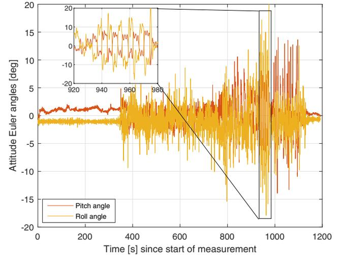
Fig. 7. Roll and pitch angle of UAV during test flight. The enlarged section refers to a period with higher pitch/ roll angle dynamics of up to  $\pm 20^\circ$ .
