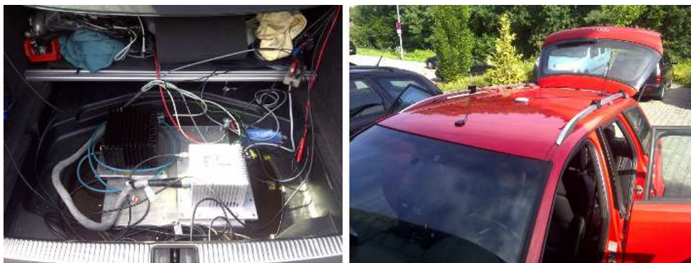
Fig. 8 Measurement equipment: The left picture shows the iTraceRT-F400 and iTraceRT-F200 of iMAR mounted in the rear trunk. The right picture shows the roof with the white Novatel antenna and the two smaller u-blox antennas in the front and at the rear. The baseline length between both u-blox receivers was 1.078m
