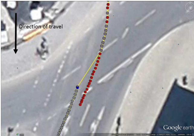
Fig. 11. Benefit of VPU - first approach at Königsplatz: The VPU-based positioning enables an instantaneous correction of the biased GPS-only and tightly coupled solutions.
