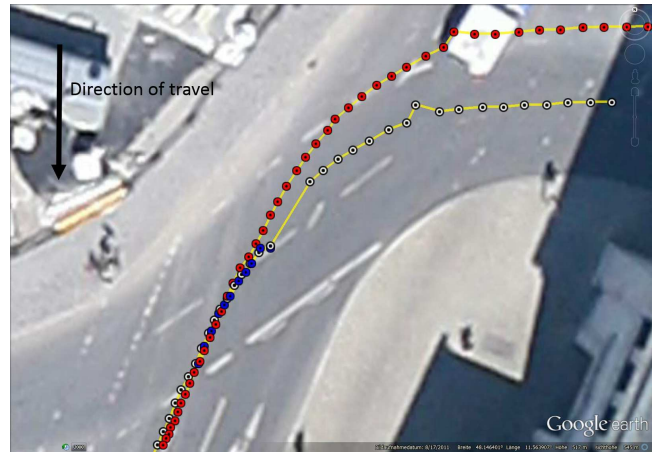
Fig. 13. Benefit of VPU - third approach at Königsplatz: The VPU provides a continuous position information over multiple epochs.
