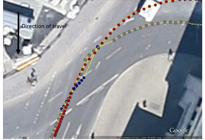
Fig. 12. Benefit of VPU - second approach at Königsplatz: The VPU is tracking a street marker over several epochs which results in a continuous position information. Only the first epoch of the VPU-based position is erroneous as the street marking is still quite far away.
