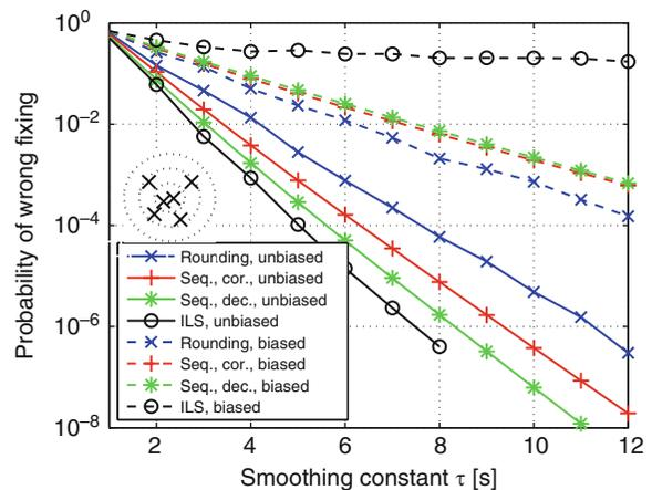
**Fig. 116.2** Comparison of integer estimation methods for unbiased and biased measurements
