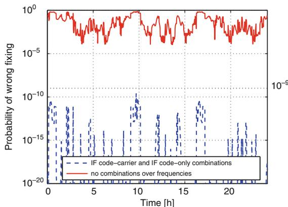
**Fig. 116.1** Benefit of multi-frequency mixed code carrier linear combinations for ambiguity resolution: the increase in wavelength from 19.0 cm to 3.285 m enables a substantial reduction in the probability of wrong fixing
