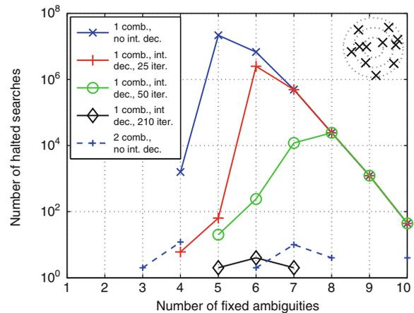
**Fig. 116.3** Reduction of halted searches by multi-frequency linear combinations
