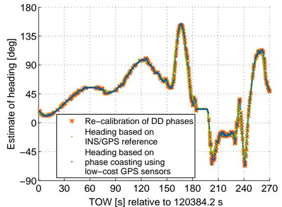
Fig. 6. Comparison of heading of proposed low cost cascaded system and of a high precision INS/GPS coupled reference system for a high vehicle speed: The heading of the low cost solution is again closely following the INS/GPS solution without a single outlier.
