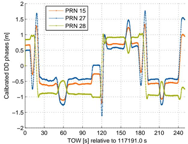
Fig. 2. Calibrated double difference carrier phase measurements correspond to the difference of two distances, which refer to the lengths of the baseline vector projections into the direction of two satellites. The noise of the double difference carrier phases lies in the order of 1 cm. Rapid changes of these double difference carrier phases indicate turns of the vehicle.
