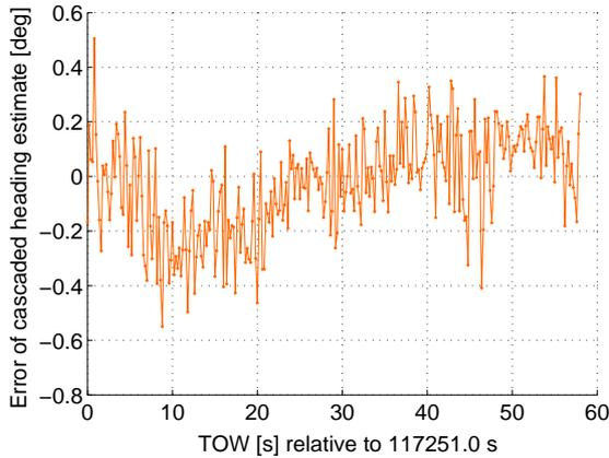
Fig. 4. Difference between heading estimates of ANAVS's low cost GPS phase-only solution and a precise INS/GPS reference system over 1 minute: The difference is close to a white Gaussian noise process with a standard deviation of  $0.18^\circ$ , which corresponds to the double difference phase noise.
