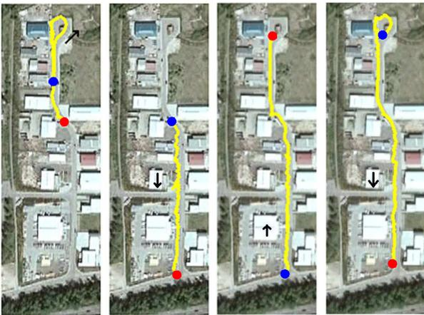
Fig. 1. Path of vehicle in urban environment in sections of 60 s with starting points marked in blue (first: TOW = 117191.0 s) and ending points marked in red: a road aligned in north-south direction was driven multiple times with turns at both ends. The shown path is based on the code measurements, which are severely affected by multipath. The much more precise carrier phases were used to determine the heading, which is shown in Fig. 3.
