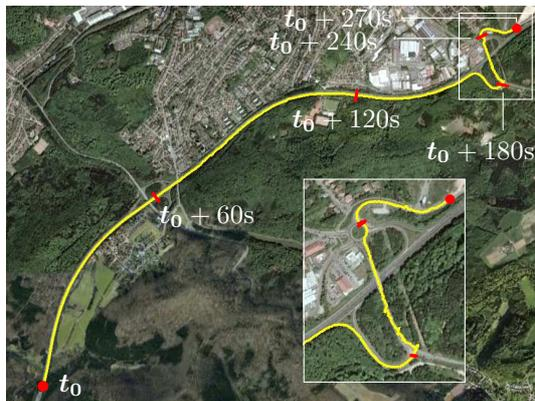
Fig. 5. Path of vehicle in rural environment with start at TOW = 120384.2 s: In the first 150 s, the vehicle was driving on a highway with a speed of around 110 km/h. The subsequent 120 s include a stop at the highway exit (180 s) and the driving through a roundabout (240 s).
