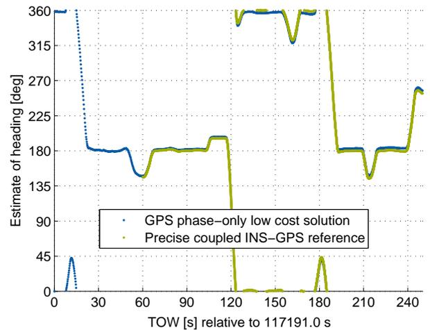
Fig. 3. Comparison of heading estimates of ANAVS's low cost cascaded system using phase coasting with an INS/GPS coupled reference system for the track of Fig 1: Both heading estimates match to a high degree.
